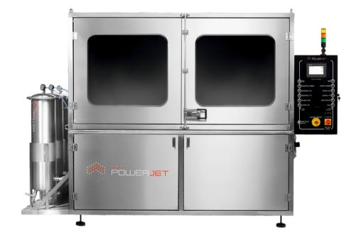
An innovative device of high efficiency utilising the hydrodynamic method of regeneration. The operating chamber allows for loading even the largest systems and all sizes of filters. Perfect workmanship in every detail guarantees trouble-free use for many years.
